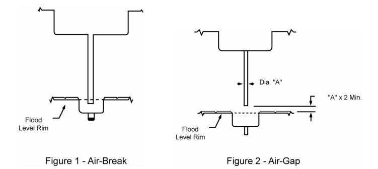
**Backflow** — The flow of water or other liquids, mixtures, or substances into the distribution pipes of a potable supply of water from any source or sources other than the potable water supply. Back-siphonage and back-pressure are forms of backflow.
