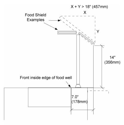
Figure 7 Sneeze Guard Detail
