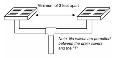
FIGURE 10a - Dual Drain System
